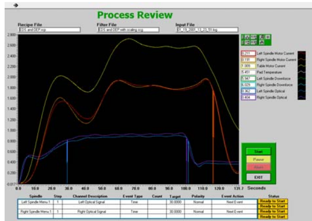
Figure 1. nVision End Point signals
